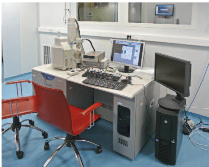
Fig. 12. Nanolithography facility fitted to a Scanning Electron Microscope (SEM) set in to function in the class 1000 section of the NIMP cleanroom
