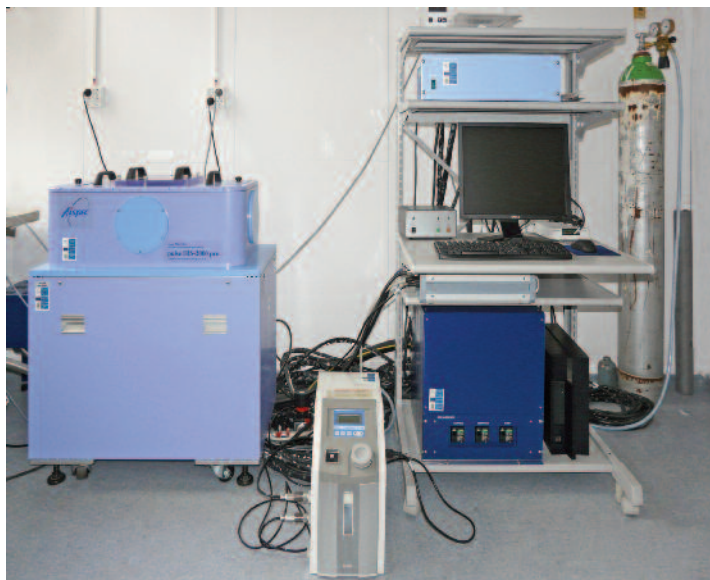
Fig. 10. TerraHertz time domain spectrometer (Aispec pulse IRS2000 pro)
