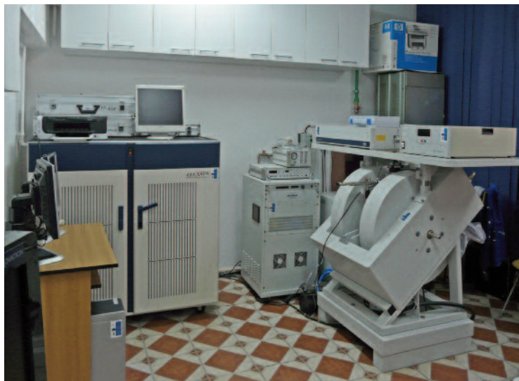
Fig. 8. Pulsed Fourier Transform X-band electron spin resonance (ESR) spectrometer model Bruker BioSpin ELEXSYS 580 10/12
