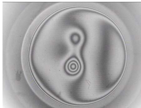
Fig. 15 – Three linear actuators without reference fringes acting on the liquid mirror.
