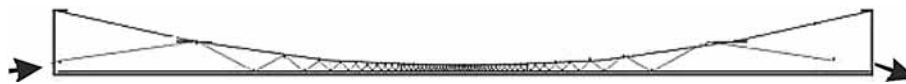
Fig. 10 – Yb:YAG/YAG microchip laser: side view of the ray propagation inside of the microchip (ray hits first the spherical surface).
