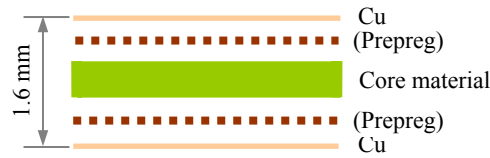
Fig. 1 – Compact different layers of the PCB substrate materials.
