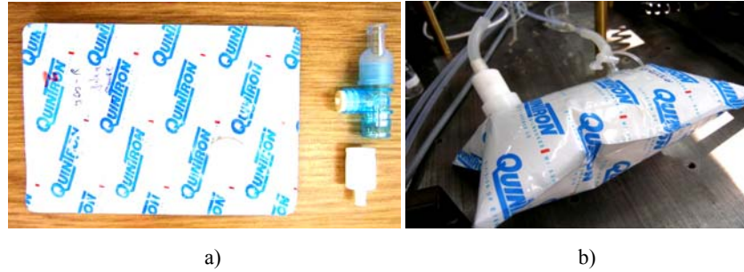
Fig. 2 – a) Chemically inert aluminized bags with mouthpieces in the right hand side and b) aluminium-coated plastic bag filled with the sample gas and connected to the PA system.
