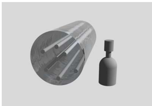
Fig. 1 – A schematic representation of the Madera measurement geometry with the calibration drum.
